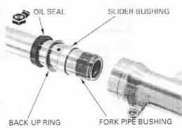
Drive the oil seal in using the special tools.
