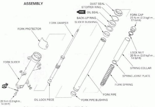
Before assembly, wash all parts with a high flash point or non-flammable solvent and wipe them dry.
