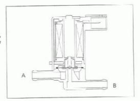
Check the resistance between the terminals of the EVAP purge control solenoid valve.
