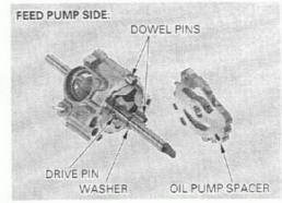
Install the drive pin into the hole in the pump shaft.
