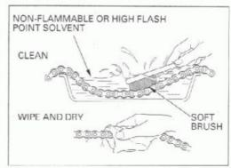
Lubricate the drive chain with #80-90 gear oil or Pro Honda chain lube designed specifically for use with O-ring chains. Wipe off any excess oil or chain lubricant.
