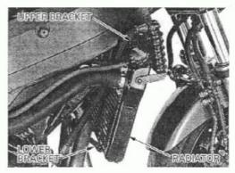
Install and tighten the radiator mounting bolt. Connect the fan motor sub-harness 2P natural connector.
