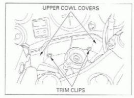
Remove the windscreen upper end special holts/ cap nuts.
