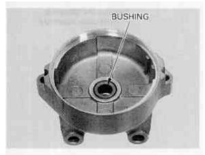
Check the front cover oil seal for fatigue or other damage.
