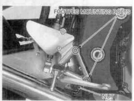
Tighten the rear master cylinder mounting bolts to the specified torque.
