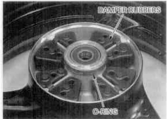
**Driven flange bearing removal**
