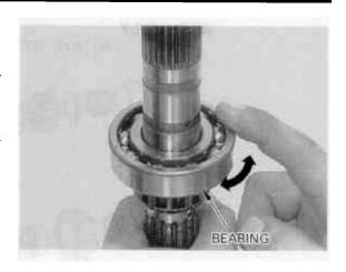
Press out the mainshaft from the bearing using a hydraulic press.
