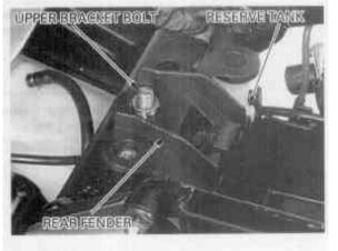
Release the rear fender from the seat rail, then remove it backward.
