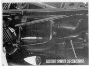
Lift the rear end of the fuel tank.
