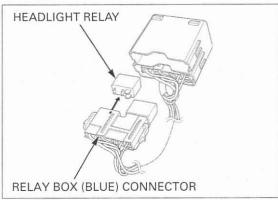
Connect an ohmmeter to the following headlight relay terminals.
