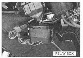
Remove the relay box (Blue) connector from the relay box, and then remove the headlight relay.
