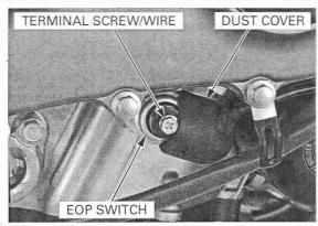
Short the EOP switch wire to ground using a jumper wire.
