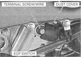
Apply sealant to the EOP switch threads as shown.
