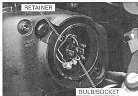
Remove the headlight bulb from the socket.
