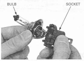
Install the new headlight bulb/socket aligning its tab with the groove in the headlight unit, and hook the bulb retainer properly.
