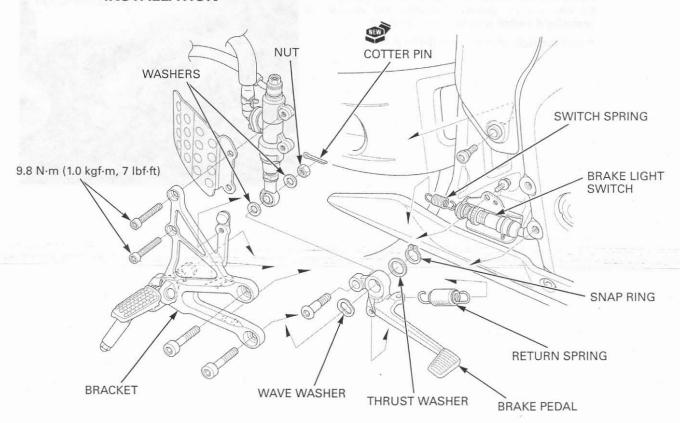
Apply grease to the sliding surface of the brake pedal and pivot shaft.
