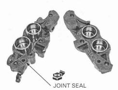
Assemble the caliper halves.
