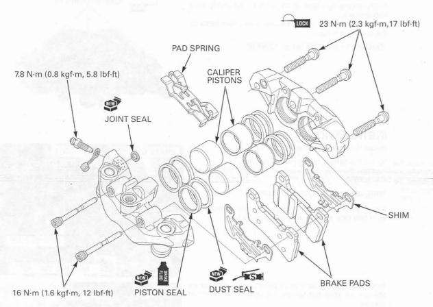
Coat new piston seals with clean brake fluid. Coat new dust seals with silicone grease.
