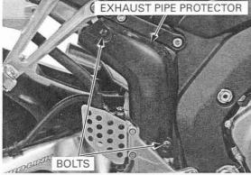
Drain the rear hydraulic system (page 16-7). Remove the bolts and passenger peg bracket.
