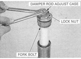
bolt after installing the fork slider into the fork bridges.
