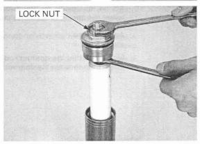
Hold the damper rod adjust case, and then tighten the lock nut to the specified torque.
