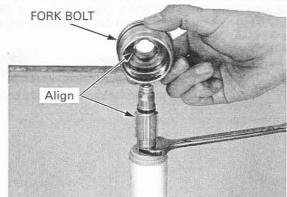
Install the lock nut to the damper rod adjust case. Hold the damper rod adjust case and tighten the lock nut.
