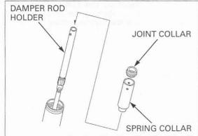
Attach the handle to the damper rod holder, then lower the spring collar while pulling up the damper rod holder.
