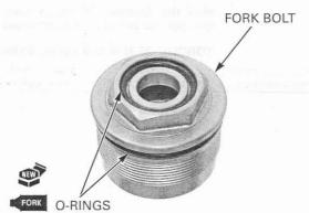
Turn the pre-load adjusting plate clockwise until it seats lightly.
