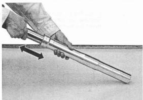
Remove the fork tube bushing, slider bushing, backup ring, oil seal, stopper ring and dust seal from the fork tube.
