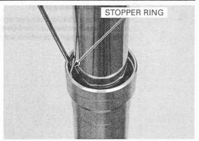
Pull the fork tube out until you feel resistance from the slider bushing. Then move it in and out, tapping the bushing lightly until the fork tube separates from the fork slider.
