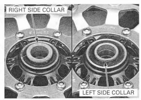
Install the front wheel between the fork legs. Apply a thin layer of grease to the front axle surface. Install the front axle from the left side.
