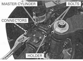
Remove the screws and left handlebar switch.
