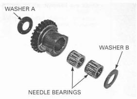
Remove the balancer gear assembly from the balancer weight.
