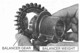
Remove the damper rubbers from the balancer gear.
