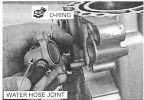
Install the water hose joint to the crankcase, tighten the two bolts securely.
