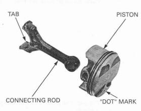
Install the piston pin and secure it using new piston pin clips.
