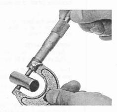
Measure the diameter of the piston at 4.0 mm (0.16 in) from the bottom and 90 degrees to the piston pin hole.
