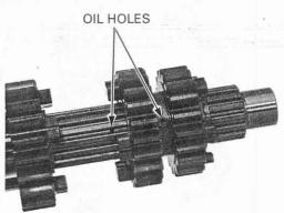
Align the oil holes between the shaft, gear and collar.
