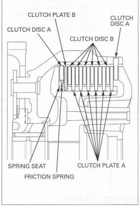
Install the clutch disc A (larger I.D. disc) and set the tabs of it in the shallow slots of the clutch outer.
