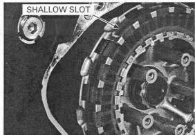
Install the push rod and clutch lifter piece into the mainshaft.
