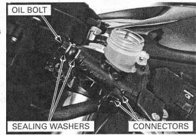
Remove the bolts from the master cylinder holder and remove the master cylinder assembly.
