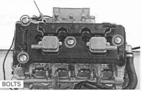
Install the direct ignition coils and connect the ignition coil connectors.
