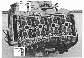
Install the cam chain over the cam sprockets and then install the intake and exhaust camshafts.
