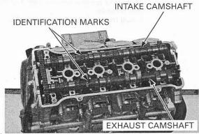
Make sure that the timing marks on the cam sprockets are facing outward and flush with the cylinder head upper surface as shown.
