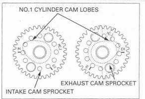
Clean and apply a locking agent to the cam sprocket bolt threads. Install the cam sprockets and bolts.
