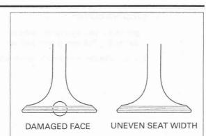
The valves cannot • Contact area (too high or too low) - Reface the valve seat.
