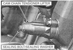
Turn the tensioner lifter shaft fully in (clockwise) and secure it using the special tool to prevent damaging the cam chain.
