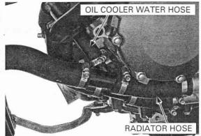
Connect the upper radiator hose to the thermostat housing cover and tighten the clamp screw securely.
