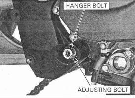
The front hanger Install the distance collars, right front engine hanger bolt is hollow. bolt and middle engine hanger bolt.
