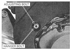
Install the rear lower engine hanger bolt from the right side.
