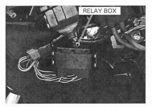
Release the retainers (brown) and remove the relay connector base.
