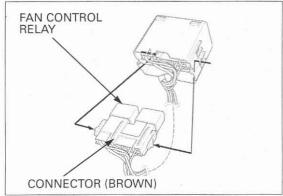
Connect the ohmmeter to the fan control relay connector terminals.
