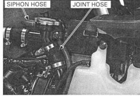
Route the radiator Install the air guide/reserve tank lower bracket onto drain hose and over the radiator, tighten the bolts securely.
