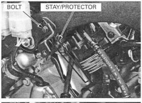
Connect the servomotor 6P (Natural) connector. Install the removed parts in the reverse order of removal.
