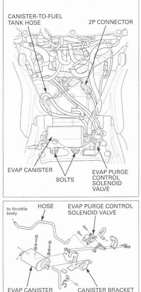
Disconnect the purge control solenoid valve-tothrottle body hose from the solenoid valve. Remove the bolts and canister bracket/solenoid
