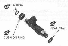
Install the fuel injectors into the fuel rail, being careful not to damage the O-ring and cushion ring.
