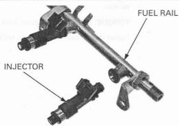
Remove the seal ring, O-ring and cushion ring.
