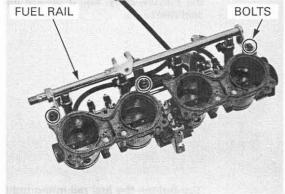
Remove the injectors from the fuel rail.
