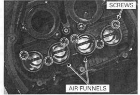
Install the upper air cleaner housing and eight screws.
