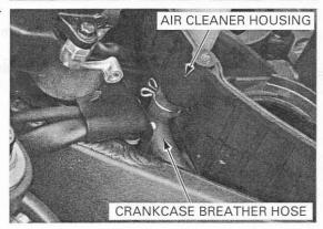
Remove the oil separation chamber from the lower air cleaner housing.
