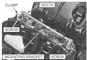
Remove the eight screws and upper air cleaner housing.
