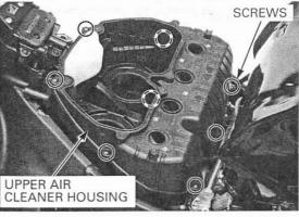
Remove the air funnel/air cleaner housing mounting screws, then remove the air funnels.
