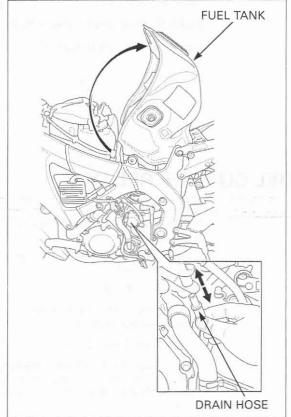
Support the fuel tank using a suitable support.
