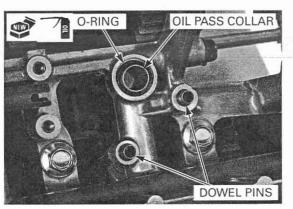
Install the oil pump assembly onto the crankcase while aligning the oil pump shaft lug with the water pump shaft groove by turning the oil pump shaft.
