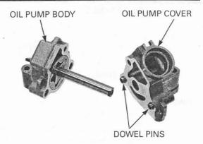
Install and tighten the oil pump assembly bolts to the specified torque.
