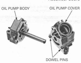
Remove the thrust washer, drive pin, oil pump shaft, outer rotor and inner rotor from the oil pump body.
