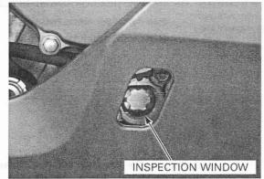
If the level is below the lower level line, remove the oil filler cap and fill the crankcase with the recommended oil up to the upper level line as follows:
