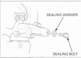
Turn the tensioner lifter shaft fully in (clockwise) and secure it using the special tool to prevent damaging the cam chain.
